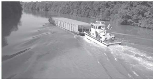
FIGURE 1. Pusher tug and barge on Rhone River, travelling upstream with approximately V_r = 4.2 m/s.
